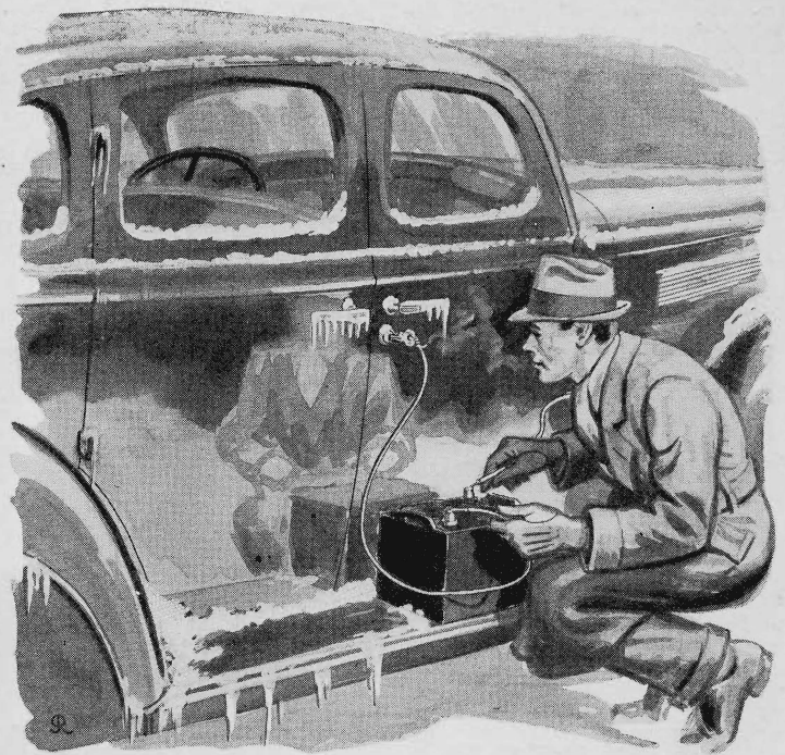
How a storage battery wired to a key can be used to thaw the ice in a car-door lock
