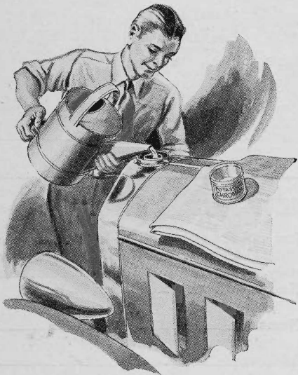
A solution of potassium chromate in distilled water guards new radiators against corrosion
