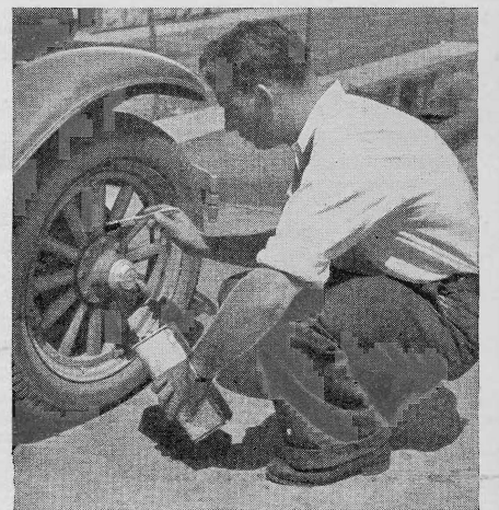
Squeaking of wood wheels, caused by dryness, can be stopped by brushing on as much hot linseed oil as possible
