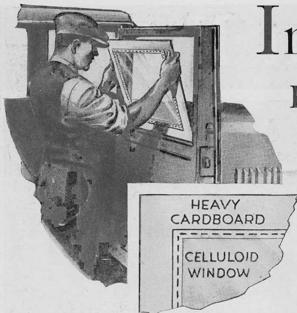
An emergency window can be made of cardboard and sheet celluloid and installed to replace broken glass, as shown above
