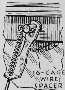
Wire wound around blade arm of windshield wiper, makes blade touch glass
