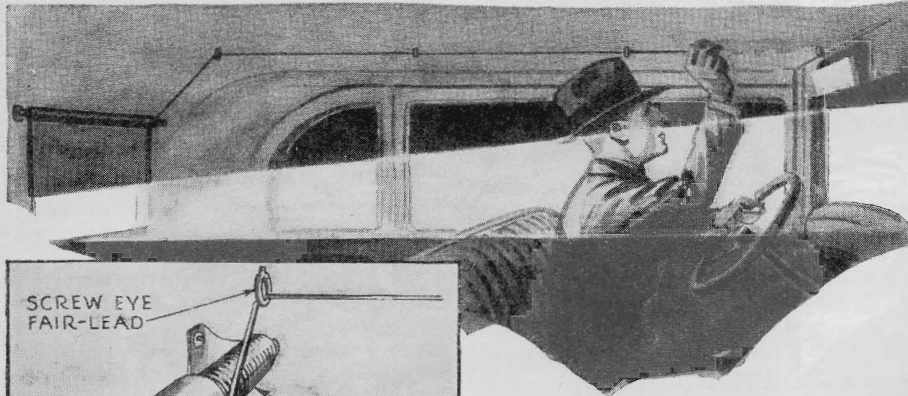
Wire, attached to car's rear window curtain roller, passes through screw eyes to driver's seat and is a means of adjusting the curtain
