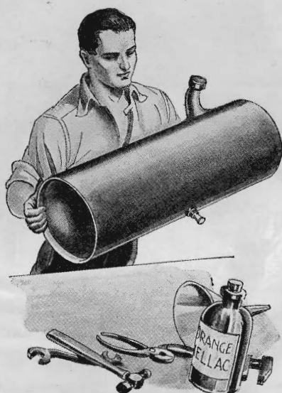
Draining the gas tank, letting it stand until dry, and then coating with shellac stops leaks.
