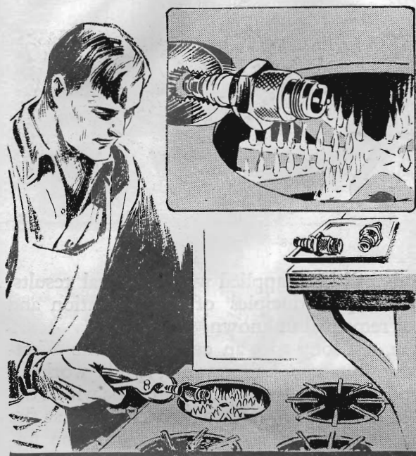
Fig. 1. Slowly heating a spark plug until it is red-hot and then letting it cool gradually will remove carbon and won't hurt plug.
