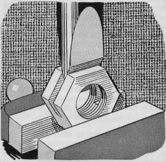
A nut that keeps working loose can be made to lock on by cutting three-quarters of the way through it, then driving a cold chisel down the groove to expand it, say, a third of a thread width. This puts tension on the threads when the nut is refitted.
