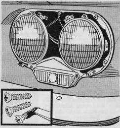
Simple maintenance can keep headlight retaining screws from rusting tight—merely coat the threads with grease. Treat the trimring screw, too, before refitting. Loosen already badly rusted screws with penetrating oil, and replace them with new ones.
