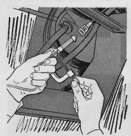
Inserting fuses in tight places is easy with a small C clamp. Pull the wire to compress the fuse-holder spring, attach the clamp to the wire to hold the spring down, and insert fuse. Twist the two pieces of the fuse holder together and remove the clamp.
