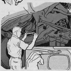
To start a cap screw where it's impossible to both hold and turn it with your fingers, drill a blind hole into the center of the head and bend up a stiff wire to fit it. Steer the screw with the holding tool while turning the cap with an open-end wrench.
