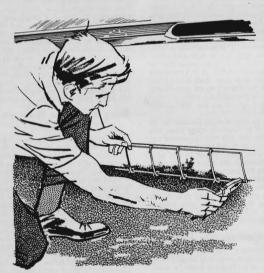
When rocker panels rust out, replacements are costly for all cars and hard to get for imports. Here's a way out. Bend some coat-hanger wire to the exact shape of the panel and take the pattern to a sheet-metal shop. They can fabricate a rocker panel quickly and inexpensively.
