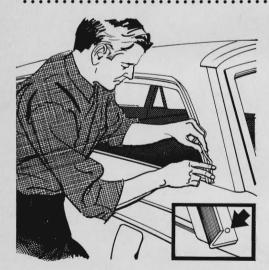
When an annoying wind whistle develops along the front or rear roof areas of a car or station wagon, check the outside drip moldings. Look for a small opening in the end or under the drip rail. The whistling is caused by air passing over the cavity and the remedy is to fill it. A little caulking compound makes a permanent repair.
