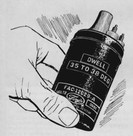
You won't forget the setting for your ignition points any more if you punch the specifications on a piece of "Dymo" tape and stick it on the coil where they can easily be read. Other reminders can be made up and stuck in proper places in the garage as well as in the car.
