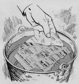
Coolant containing antifreeze, drained and stored in a bucket or a can during a repair job, ends up with a film of oil over it. Remove this film before refilling the radiator by placing a sheet of newspaper on the coolant surface—it will readily absorb the oil. A discarded desk blotter will do the job nicely, too.
