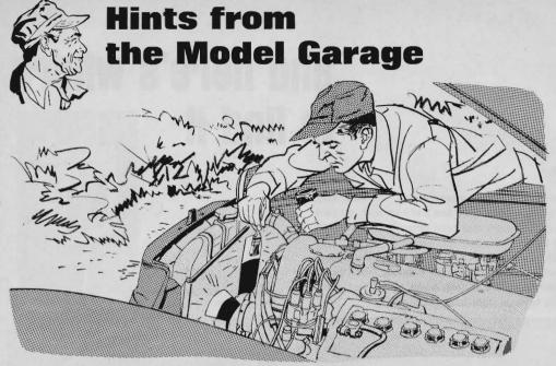
Working under the hood of a car while the engine is running — as it must for some checkup and repair operations — can be dangerous. Absorbed in your work, you can forget to keep your fingers out of the way of the revolving fan —
