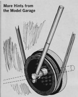
To turn an engine to an exact point, the best way is to mount a socket and sliding T handle on the bolt that fastens belt pulley to crankshaft. Use a long handle to get lots of leverage for large-displacement engines. The handle makes it easy to work without hitting connections.
