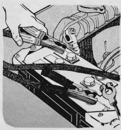
Disconnect both battery cables when boostcharging your battery. Otherwise, you may damage transistors, diodes, and rectifiers used in clocks, impulse tachometers, radios, and alternators. Semiconductors can be damaged by "foreign" currents exceeding their own ratings.
