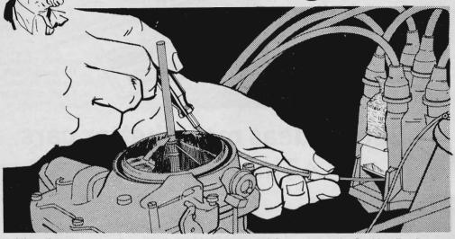
Holding the trapdoor of a distributor open when you're adjusting the contact points externally can be difficult on late-model General Motors cars with Delco distributors. Here's an easy way to get around the problem: Use masking tape. It does a good job of holding the trapdoor
