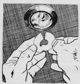
Old dome-light reflectors are often dull, flaked, or tarnished. Fix yours by cutting a small piece out of the bottom of a store-bought aluminum pie pan, slip this under the bulb bracket, (shiny side down), and refit the glass. A double-folded piece of aluminum foil also works.
