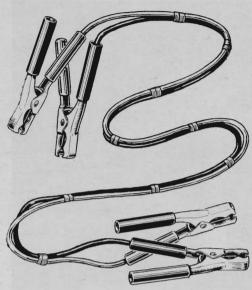
Battery jumper cables won't get tangled if you tape them together at short intervals. Be sure to leave about 18" free at each end to allow the cables to be hooked up easily. After they're used, they can be coiled up neatly and easily for storage.
