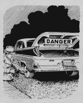
A hinged reflective sign hanging from the trunk lid can save your life when you make emergency repairs at night. It's made of a 4'-by-8" piece of ¼" plywood with red reflecting-tape letters. A cupboard door catch holds it up against lid till needed.
