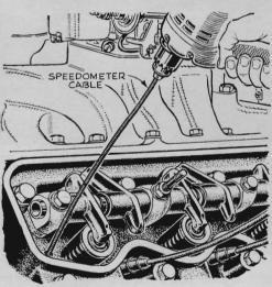
Clean out clogged oil-return ports in OHV engines with a piece of discarded speedometer cable inserted in a power drill. The digging action often does the job where air pressure fails. Don't press too hard, or the cable may kink and fray.
