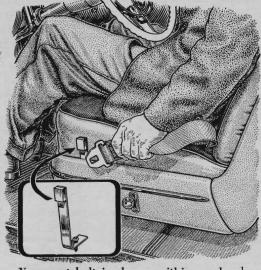
Your seat belt is always within reach when you secure the short end with this holder. Cement a small magnet to a ½"-by-4" steel upright. The right-angle bend in the upright holds it snugly between seat frame and cushion. Bolt it if necessary.
