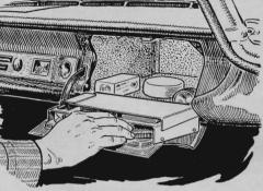
To keep your glove box neat, make this dual-compartment container from sheet copper and mount it on the inside of the lid. Roll the front edges for safety. The dimensions given are for 1958-62 Ramblers, but they can be changed to fit other cars.
