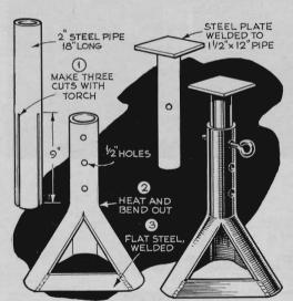
Car supports are easy to make with 2" pipe. Cut three slits with a torch, heat, and bend strips out to form a tripod. Brace with flat steel. A piece of 1½" pipe with a platform welded on is adjusted with a ½" pin inserted through one of three holes.
