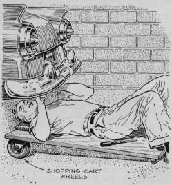
To make a creeper more maneuverable while you're working under a car, replace the small casters at the front (pillow end) with larger wheels. A pair of swivel wheels like those on a shopping cart can be adapted easily for this purpose.
