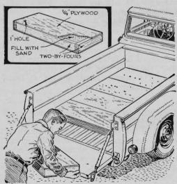
Need ballast in your pickup truck when it snows? Five of these sandboxes take up little space, and they won't slide around. Tops and bottoms are ¼-inch plywood; sides are two-by-fours. A one-inch hole in the top of one lets you use sand on ice.
