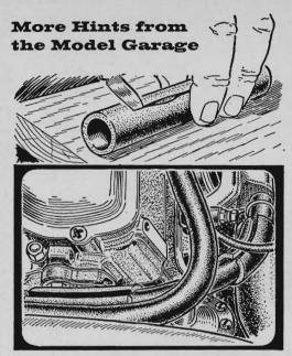
Installing new heater hose? Don't junk the old one. Cut it into short sections, slit it lengthwise, and slip it over the new hose at all points where it may wear against the oil lines or battery case. It will stay on without fastening.
