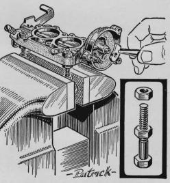
Securing a carburetor in a vise is necessary at times for repairs. To hold the carburetor firmly without damaging it, clamp two 3/8" bolts in the vise. Then bolt the carburetor to them through the mounting holes in the flange.
