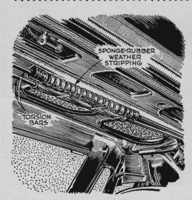
Noise under the deck lid on some cars may be due to rattling of the torsion bars that hold the lid up. If they hit against each other, wrap one rod with spongerubber weather stripping. Ends can be fastened with electrician's tape.
