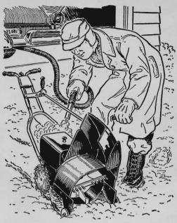
Small four-cycles start faster in cold weather if warmed by a car's exhaust. Attach an old vacuum-cleaner hose to the car's tailpipe, and play heat around the engine cylinder and intake of your snow blower, tractor, or other machinery.
