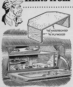
A glove-compartment shelf lets you make better use of limited space by filing road maps up out of the way. It's easily made of ½" hardboard with ½" plywood for the supports. Make a cardboard pattern first to insure proper fit.
