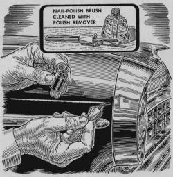
Touch up paint chips and scratches with a nail-polish brush. It's just the right size and its handle is conveniently shaped for detail work. First clean the brush with polish remover. Promptly taking care of chips prevents rusting and blistering.
