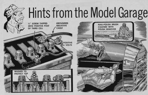
Tapping a 12-volt battery is cheaper than buying a resistor when six-volt current is needed for electric brakes on trailers. Drill a hole in the positive post of the third cell and install a 4" screw to act as a terminal for the six-volt cable lead.
