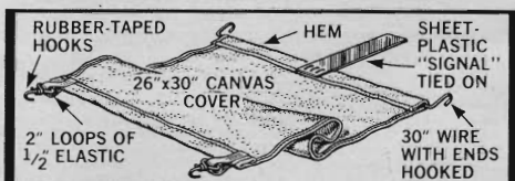
"SIGNAL" SEEN IN REAR-VIEW MIRROR IF COVER IS LEFT ON
