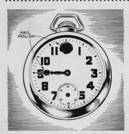
To avoid parking tickets, convert an old watch into a parking-meter timer by removing all but the minute hand and painting on red dots. Set it backwards for the time you paid for (15 minutes shown above) and check it as you shop.
