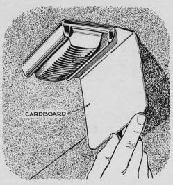
The dome light can be used by passengers in the rear seat, without reducing the driver's visibility, if a shield is placed in front of the light. Loosen the holding screws, slip folded cardboard under the frame, and tighten the screws.
