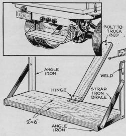
A rear step on a truck is sometimes useful, sometimes not wanted, depending on the work being done. A removable step solves the problem. Fasten it in place with hinges, using heavy cotter pins instead of hinge pins to join them.
