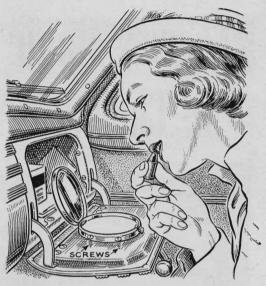
Mirror Is Always Handy. Here's the way W. M. Dierks, of Chicago, filled the bill when his wife asked for a convenient mirror for use in the car. Buying a large compact, he mounted it as shown inside the glove-compartment door, drilling holes and attaching it with screws. While not in use, the compact is kept closed.
