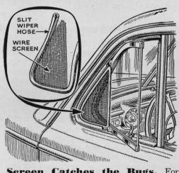
Screen Catches the Bugs. For summer driving, a triangular piece of screening fitted into the area in front of the vent pane will catch any insects that are drawn in with the air. You can solder a heavy wire around the screening or just slip on slit wiper tubing as in the sketch. It's only a moment's work to slip out the screen and close the ventilator.
