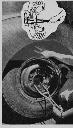
TIRE-LIFTING TOOL. Changing wheels will be easier with this two-pronged device that simultaneously supplies lifting leverage and lines up the wheel holes with the proper bolts or lugs. Prong spacing can be adjusted to suit any automobile wheel. The T. E. D. Corporation, of Los Angeles, is the manufacturer of the new wheel changer.
