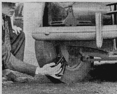
Inserted between the brake drum and rim, this one-piece jack raises the wheel off the ground when the car is driven either forward or backward.
