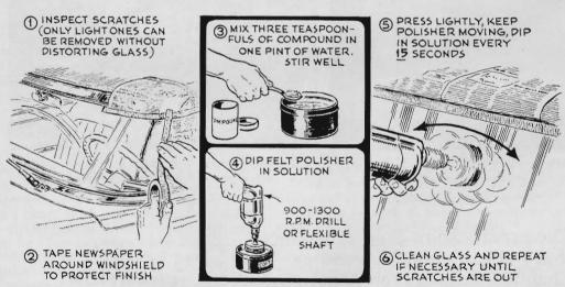
**Light scratches on a windshield** can be polished out without affecting visibility, but removal of a deep scratch might cause distortion in the glass. If the deep scratch is in the line of vision, it had best be left alone or the glass replaced. To
