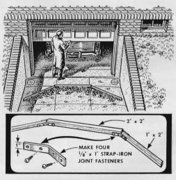
If leaves and dirt blow into a basement garage when the door is open, you can keep out most of the debris by installing a wooden barrier like this. The wheels of the car pass over the low end of the barrier without difficulty.
