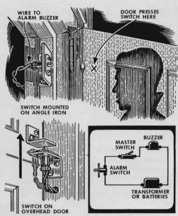
A burglar alarm is easily rigged up on a garage door with an inexpensive car courtesy-light switch connecting a bellwire circuit with a bell or buzzer in the house. A master switch wired into the circuit permits disconnecting the alarm when you open the door yourself.
