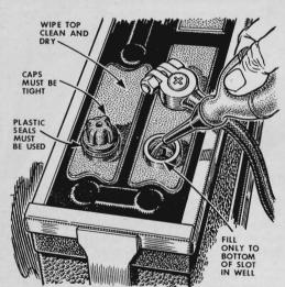
If you own a 12-volt battery, extra care is needed to control factors that cause corrosion. After careful filling, wipe off any spilled water. Corrosion is speeded by high current flow across the top of a wet battery.
