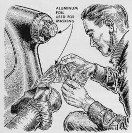
Aluminum foil can be used for masking bumper guards, bumpers, head lamps and other parts of a car when it is being spray-painted. The foil can be pressed around the parts without the use of tape. The sheets can be used repeatedly.
