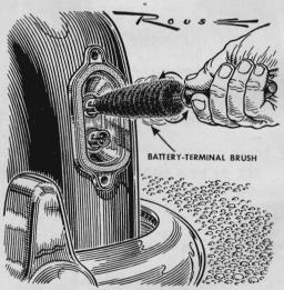
**Dirty, corroded sockets** in tail lights, small parking lights and older-type headlights can be cleaned with the end of a battery terminal brush rotated briskly inside the fixture. Turn off the switch to avoid a short.
