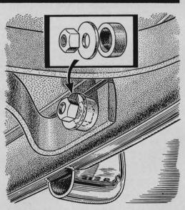
A frozen nut on a loose bumper guard can be bypassed this way on cars that have long guard bolts. Cut a short collar of pipe large enough to fit over the nut and slightly longer than the nut's thickness. Then add a new nut and washer and draw up tight against the collar.
