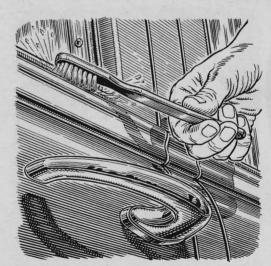
**Use a toothbrush** to remove the dried and whitened polish from body seams or behind chrome trim. The same brush can be used to *put* wax in these places as a precaution against body rust or to clean dust from the instrument panel and radio grille.
