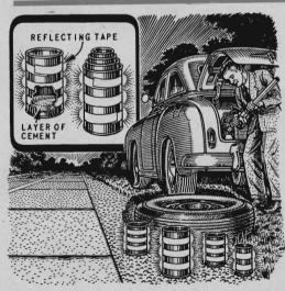
Wrap reflective tape around tin cans to warn passing motorists when you're stuck or changing a tire. Use cans of different sizes so they will nest compactly in the trunk and pour a little cement in the bottom of each can to keep them from blowing over.
