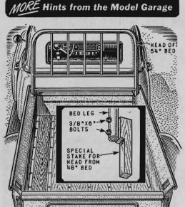
Use the head of an old metal bed to keep the load in a pickup truck from crashing through the rear window when you stop suddenly. Cut a hole in the body sides for the legs. Make the head of a narrow-width bed fit by adding wood extensions (inset).
