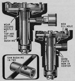
When a distributor bushing wears, play in the shaft affects engine performance. Because most wear is at the bushing ends, you can save fitting a new one if you cut the old bushing in two, drill a new oil hole and put it back with the center sections out.
