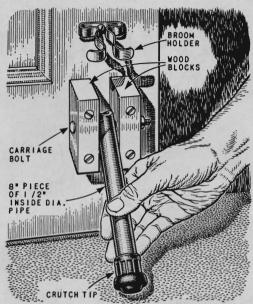
**Keep the garage door open** while you back out by pivoting a piece of pipe on a bolt held by two blocks of wood screwed to the inside of the door. A rubber crutch tip keeps it from slipping and a spring clamp stores it up out of the way.
