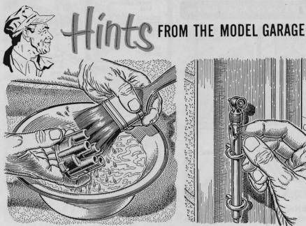
Washing the distributor cap thoroughly with white gasoline may save you the cost of a new one in the case of ignition trouble. A film of grease and dirt inside and outside the cap can cause shorts, resulting in missing and misfiring.
