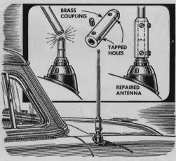
If an antenna is broken by mischievous children or overhanging tree limbs, it can sometimes be put back into service by making the repair illustrated here. The coupling might be made from a piece of brass, which makes a good electrical connection. Setscrews turned into the tapped holes will keep the two aerial sections together.
