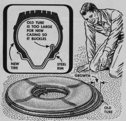
Because rubber grows in use, putting an old tube in a new tire may not be a good New tubes usually are smaller in cross section than the same size casing to allow the tube to stretch into place inside the tire. An old tube may become pinched.
