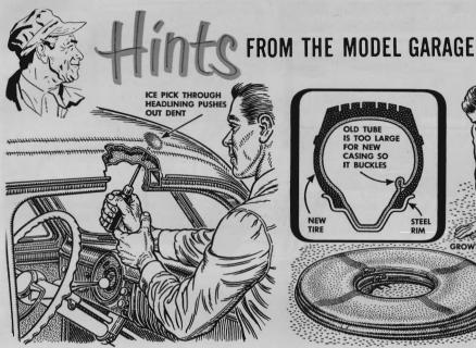
A small dent in the top of a car can often be pushed out by pressing a blunt ice pick or knitting needle through the headlining and tapping up. Then scratch the material around the hole in the headlining and fuzz it up to remove traces of the hole.
