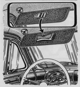
A rectangular piece of metal with one end screwed to the sunshield makes a handy clip for your sunglasses. Just slip the case on the clip. Sheet brass or aluminum might be used for the clip. Polished with steel wool, either metal will look good.
