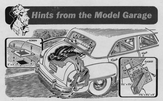
**Rear air outlets** installed like this will often increase the effectiveness of a heating system that draws fresh air from outside, especially if the car is tightly sealed. The circulating air also will help keep the side and back windows free from fog, keep the
