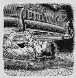
For work under a car, a gooseneck desk lamp is an excellent addition to a creeper. Drill the base of the lamp and screw it to the creeper. Invert the shade to throw light up. The flexible neck will keep the light in the desired position.
