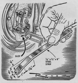
A wrench for adjusting brake shoes can be made from a piece of %" by %" by 8" mild steel. File a %" slot in the end and bend to the shape shown above. Use by inserting it in the slot on the backing plate and prying around the notched wheel.
