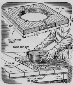
Removing the air-cleaner cover on a new Cadillac can be troublesome. Driving it off from underneath may deform the metal. This clamping device will do the job with ease. Remove the cleaner from the engine, clamp the bottom between the leather-lined jaws, and you can twist off the top without causing any damage to the metal.
