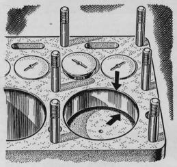
In scraping carbon from an engine during a top overhaul, some mechanics contend you can do too good a job. Their practice is to leave a ring about ½" wide around the top edge of the piston and another ring around the bore just above piston travel. This, they say, will preserve the oil seal. Removing the carbon may make the car an oil hog.
