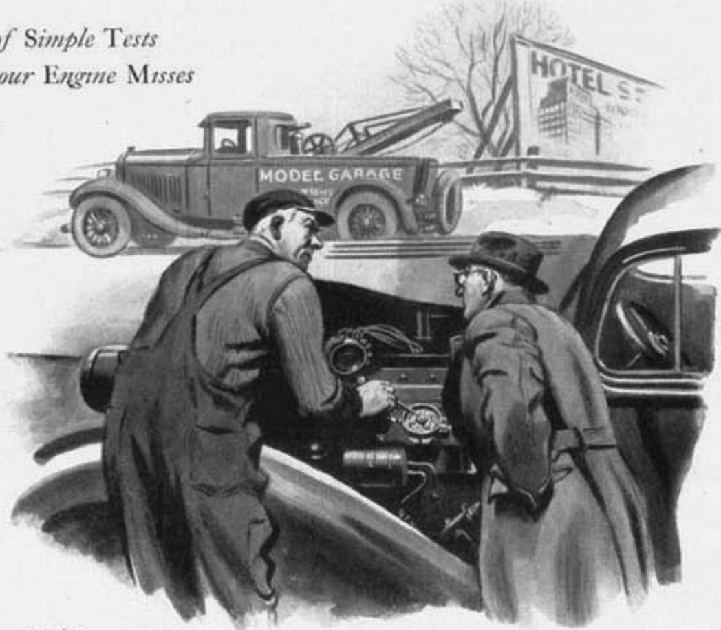
As Gus opened the distributor and bent over to inspect it, his face broke into a grin. "There you are!" he exclaimed. "The timer contact lock has worked loose, and the gap has closed up."
