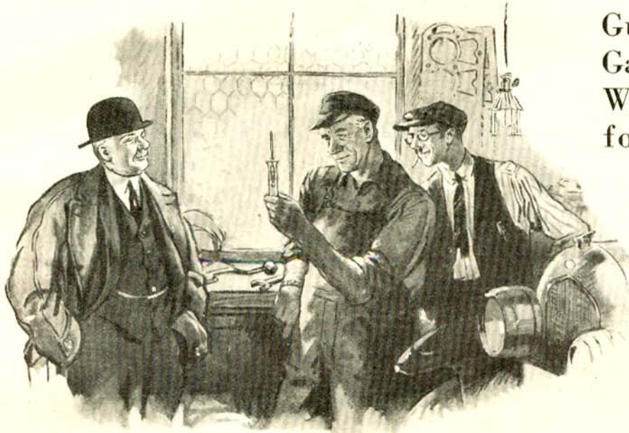
"Paste this in your hat," Gus suggested. "A glycerin solution that floats this particular hydrometer at 1,080 will keep Jack Frost out of your radiator down to ten degrees."
